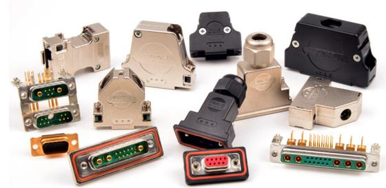
FCT Mixed-Layout D-Sub Connectors and Backshells
