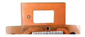
Handles of various types can be added to reduce stress on parts and installers.
