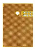
Plane layers should be designed with cross-hatch patterns to reduce weight and increase the circuits' flexibility. Cross-hatching reduces circuit thickness compared to solid ground planes. It also allows wider traces to be used, thereby increasing manufacturing tolerance and capability. Molex has successfully designed cross-hatched reference planes in high-frequency applications up to 16 Gbps.
